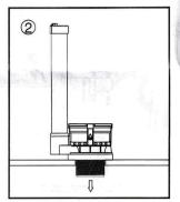
Install the base into drainer hole, adjust it perfectly to the wall if water tank, rotate it with suitable angles.
