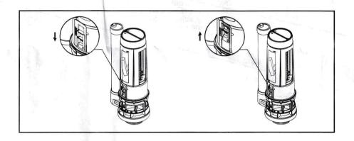
Adjust the all water controller to control its water volume, when turn it down, the button hole will close, its water volum, will be more, and vice versa.
