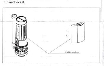
Adjust half key float to control its displacement, float is higher, its displacement will be less.
