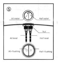
adjust the button to make the halt level aim at Half water button, all level aim at all water button, rotate
