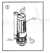
rotate the body, separate it from the base
