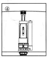
put button into the hole, rotate push rod and adjust its height to touch button.
