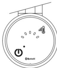
When the set time elapses, the heating element automatically returns to the settings from before the activation of the timer function. With the TIMER function active, you can freely modify the operating temperature (
