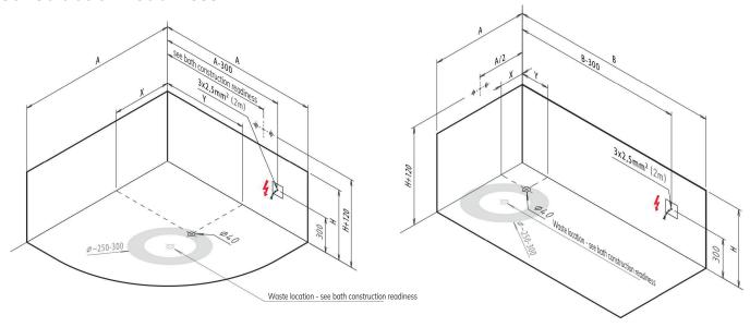
A, B ..... tub dimensions (see tub datasheet) H ..... tub height (see tub datasheet)
