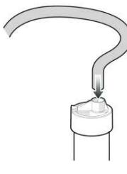
4. Attach one end of the refill tube to the overflow pipe, and the other to nipple located near top of valve.
