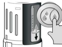
7. Press half flush button (1 water drop). Ensure that bowl empties sufficiently, and siphon action is activated. If siphon action is not activated, adjust  $\frac{1}{2}$  flush setting (blue) down one notch to 8.5. Press half flush button again. Repeat this process until the siphon action is activated.
